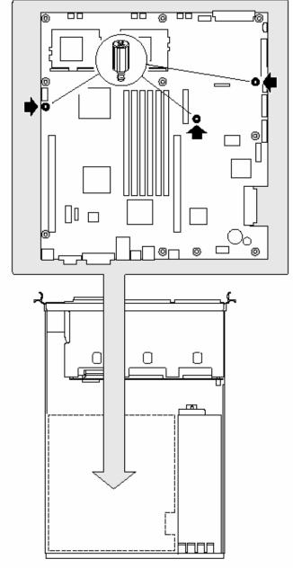
Figure 11: Attaching the Server Board
